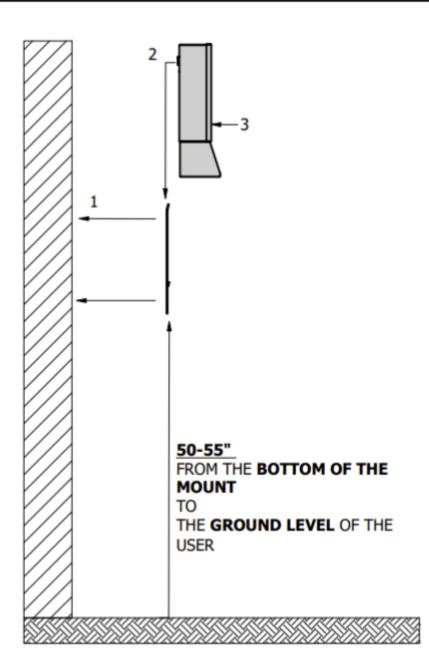
STEP 1: USING THE THROUGH HOLES ON THE MOUNTING BRACKET, SCREW THE MOUNT INTO THE WALL USING FASTENERS RATED FOR YOUR WALL TYPE (WOOD, CONCRETE, ETC.)
